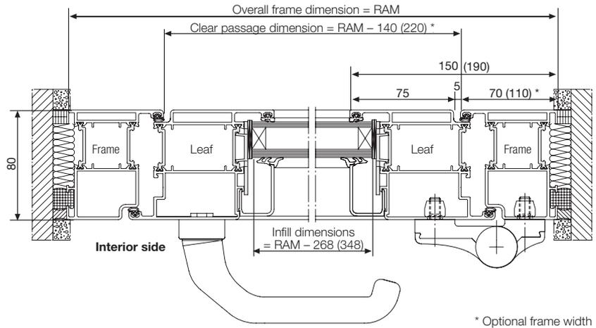
At a 90° opening angle, the clear passage is reduced to  $RAM - 214$  mm (by 294 mm with a 110 mm frame) due to the protruding leaf \*handles and levers not taken into account.
