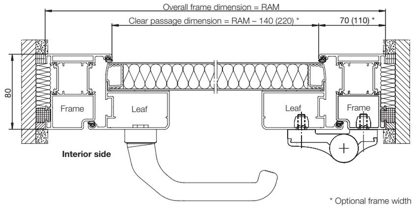
At a 90° opening angle, the clear passage is reduced to RAM - 204 mm due to the protruding leaf.
