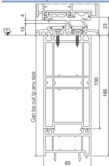
Bottom spacer profile (h = 165 mm), plastic, can be cut to length, separate, BP-K
