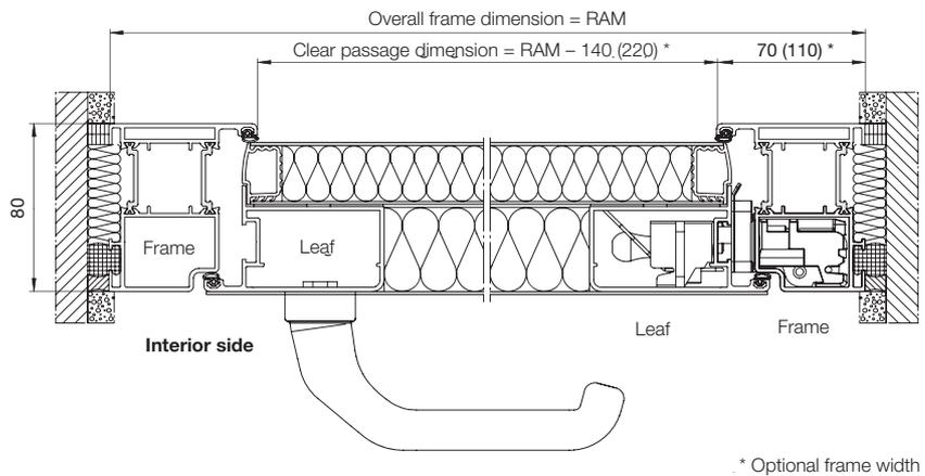
At a 90° opening angle, the clear passage is reduced to RAM - 162 mm due to the leaf overlap.
